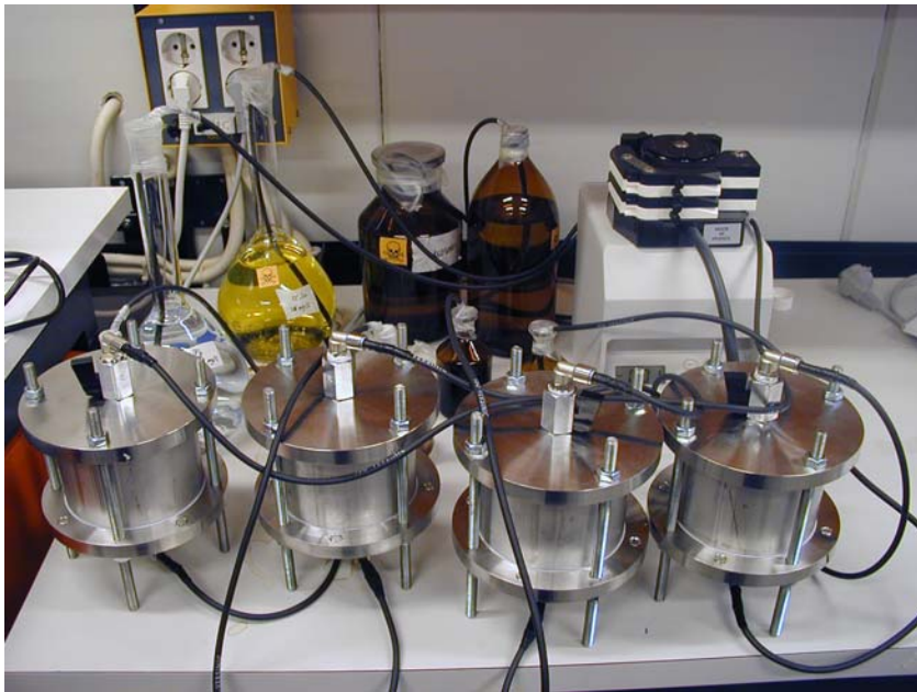
Fig. 4. The column test in progress
